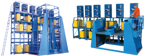
OPERATOR ABOARD BATTERY EXTRACTORS
